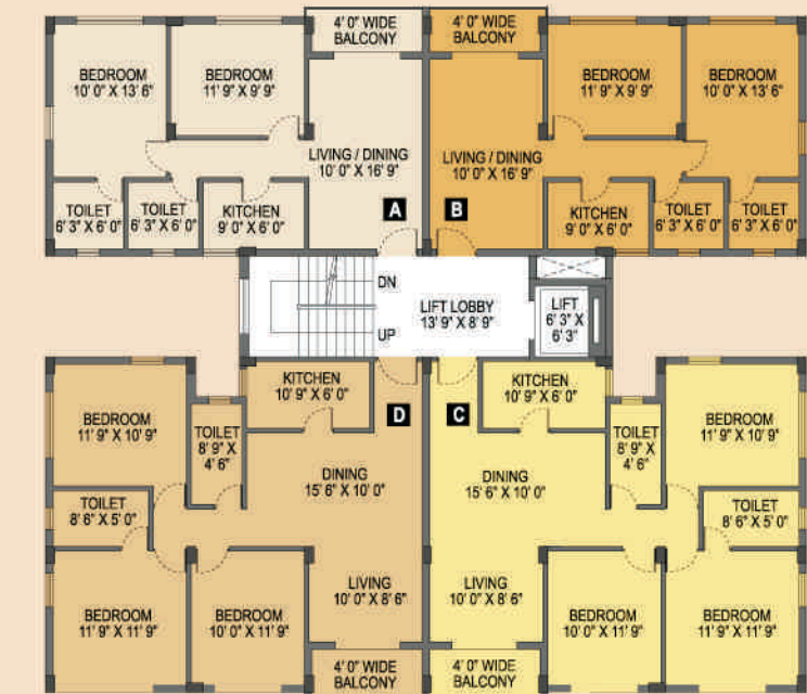
Typical Floor Plan (Block 2)
